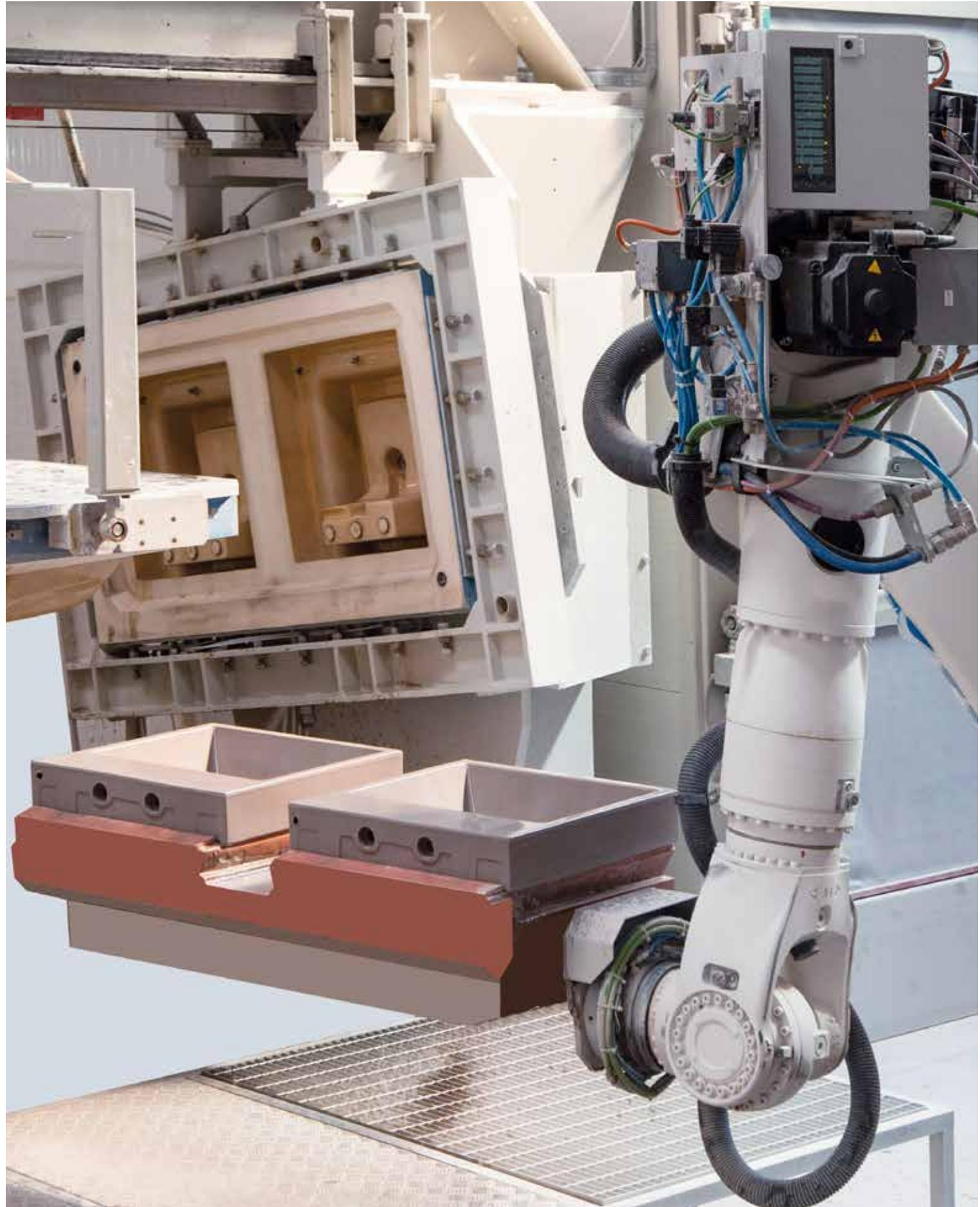
High pressure casting with split moulds
