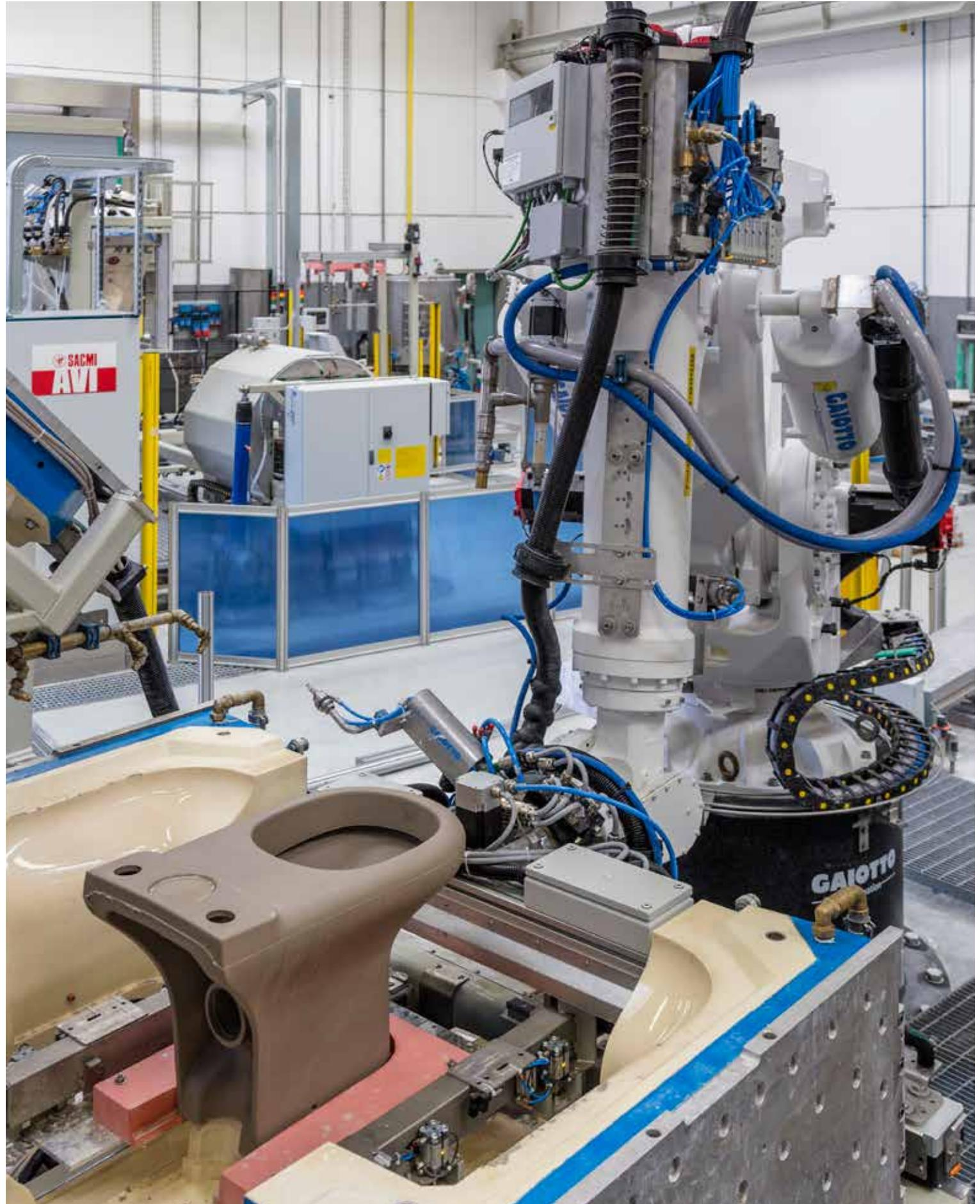
High pressure casting with multi-part moulds
