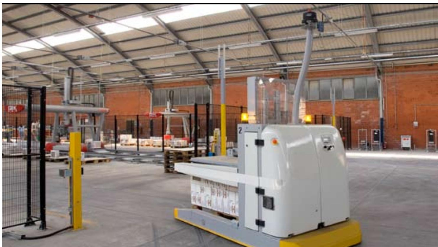
Laser guided vehicles are designed to cover any free routes without any linearity nor orthogonality requirements: loading and unloading stations can be freely arranged by making the most of the available space.
