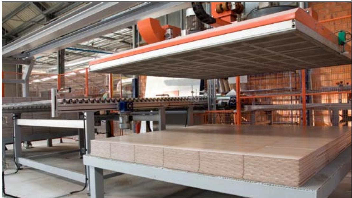
To increase tile stack stability during handling, adjacent levels can be offset so that layers can be tied.
