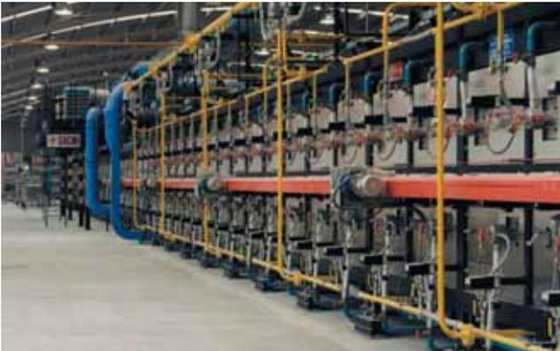
*Single-layer roller kilns directly derived from our world-renowned pressed tile kiln range are used.*
