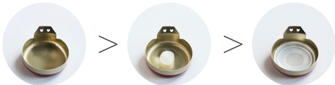
Automatic lining machines designed to extrude pellet-form material (e.g. PVC-free, PE, EVA), cut it into single doses, insert them into aluminum screw caps and mould the liner according to a clearly defined profile. Machine productivity is strongly influenced by the material type and the weight and profile of the liner.
