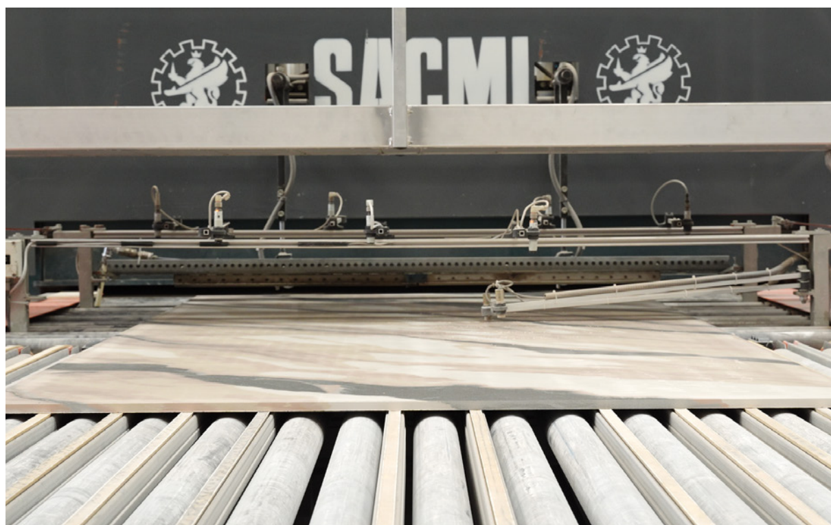
Digital tracking of the slab (Id-Tiles) - Tracking digitale della lastra (Id-Tiles)
