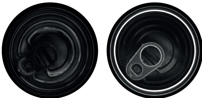
SACMI's Double Shot technology, allows the system to capture two images of the same object, under different lighting and in just under a millisecond. It is mainly applied on MVS systems for inspection of post-repair varnish on EOE lids (Double Shot UV).
